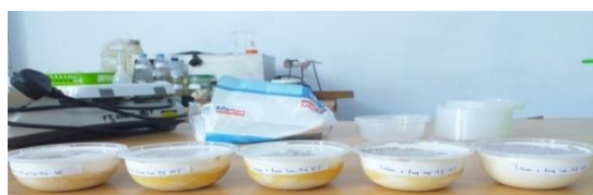
Figure 3. Latex with non-grade liquid smoke coagulant
