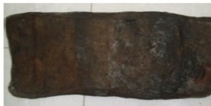
Figure 5. Latex Coagulated Using Formic Acid (Asmawit, et al, 2011)
