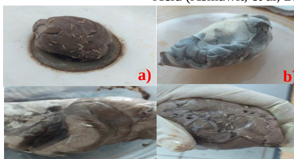
Figure 6. a) Maggots Growing on Latex Liquid Smoke Coagulation Grade III Concentration of 10% , b) non-grade Concentration of 10% c) non-grade Concentration of 25% and d) Pure Latex Without Coagulants
